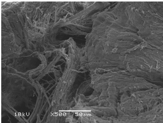
Figure 2. SEM image of the tannery solid wastes.
