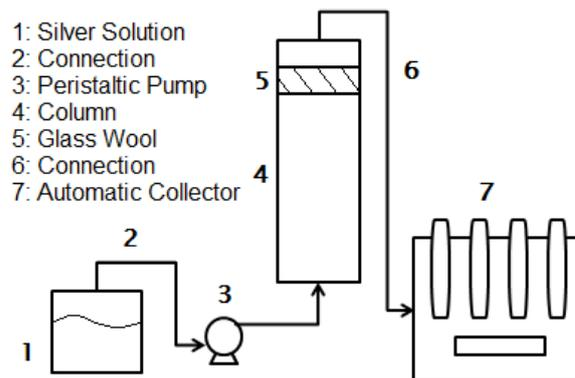
**Figure 1.** Experimental system used in this study.
