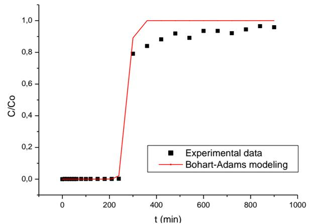
**Figure 3.** Bohart-Adams adjustments for the breakthrough curve of silver removal using a flow of 5 mL/min.
