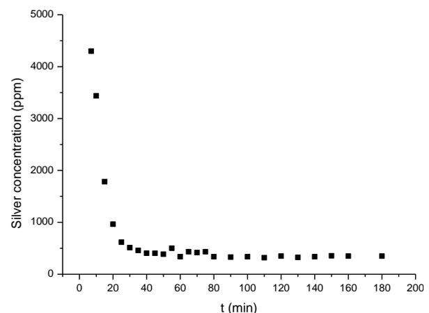
**Figure 6.** Second desorption cycle for the adsorbent's degeneration
