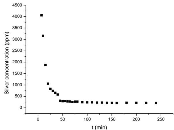
**Figure 5.** First desorption cycle for the adsorbent's degeneration
