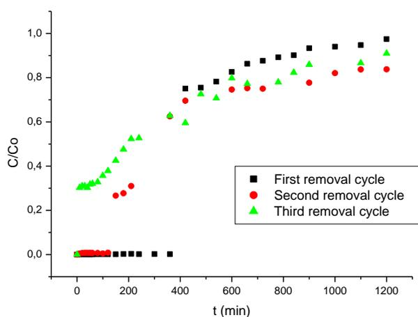
**Figure 4.** Breakthrough curves obtained for three adsorption cycles after the regeneration of the adsorbent.
