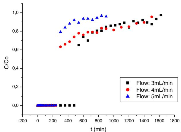
**Figure 2.** Breakthrough curves obtained for three flow rates analyzed: 3, 4 and 5 mL/min.
